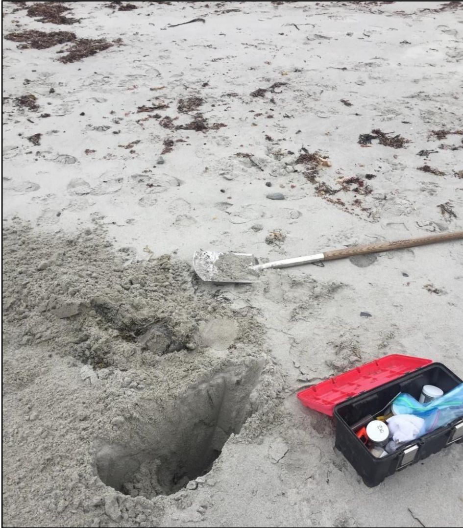
Figure 2. Sample pit from which sample BWB S1 and S2 was obtained. The pit was excavated to a depth of about 75 cm. A stainless-steel shovel was used to obtain all samples and was thoroughly cleaned between each sample site. Photo taken 1/16/2021
