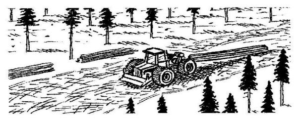
**Figure 27.** *Skidder preparing site for planting while hauling wood from harvest operation.*
