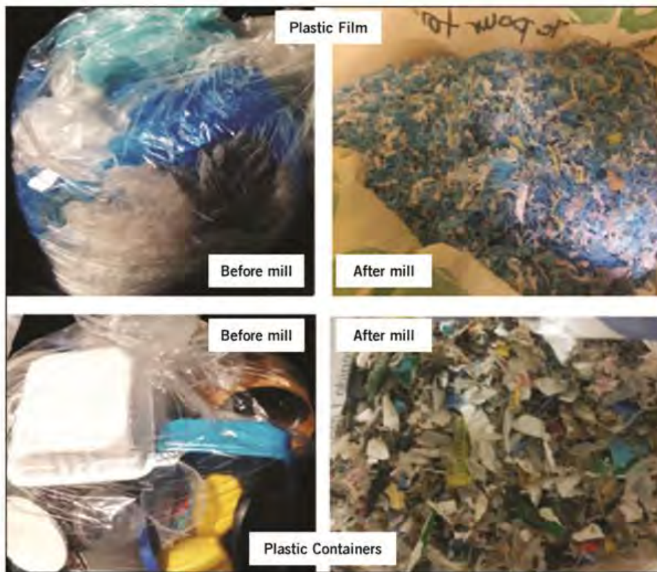
FIGURE 1: Potential sources of plastic waste derived alternative fuels before and after size reduction. Such plastic films and crushed containers contain large quantities of energy which could displace a reasonable fraction of coal/coke.
