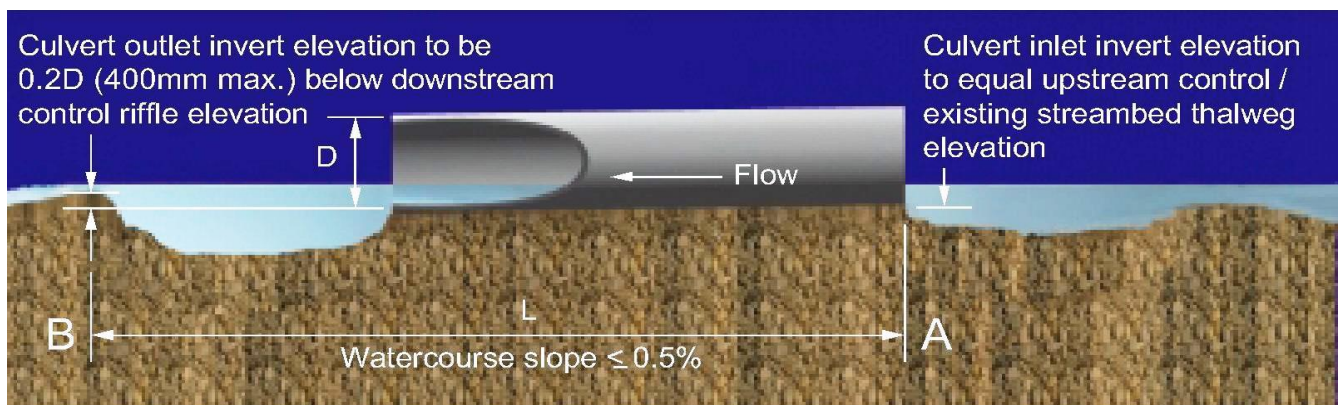
Figure 5-9 Culvert installation in watercourse with a slope equal to or less than 0.5%
